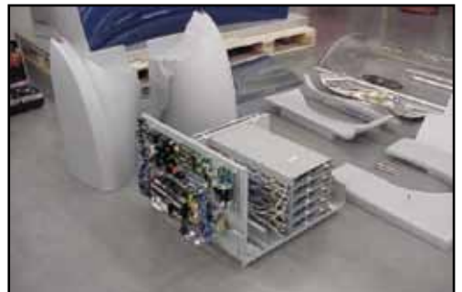
27. Disconnect plugs X3 through X8, P9A/B and P10A/B from main board. (Figure 20)
