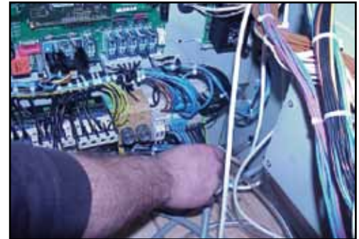
26. Disconnect the connecting lead. (Figure 19)
