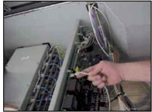
25. Disconnect the display cable. (Figure 18)
