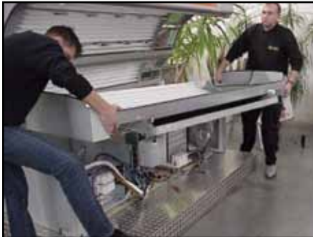
21. Lift bench to remove toward front. (Figure 15)
