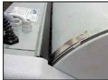
38. Loosen the canopy safety plate. (Figure 31)
