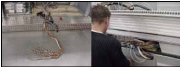
40. Gather the canopy harness and set in rear wall. (Figure 33)
