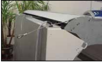
37. Pull the canopy cables upward. (Figure 30)
