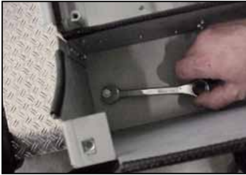
20. Remove the screws on the front left and front right from the bench section. (Figure 14)
