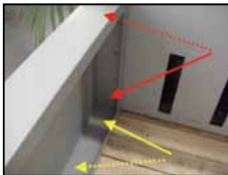
41. Lateral sections; remove the transportation safety locks and the screws that connect to the rear wall. (Figure 34)
