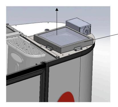
Lift the filter upwards from it's position.
