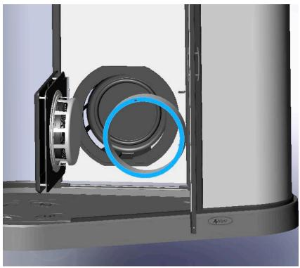
Remove the blue and white filter material. Replace or clean filter before running booth again.
