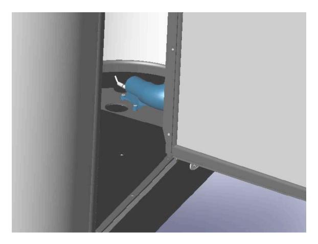
Lift drain pump panel to access sump area, clean the tub with warm water and soap. Then, wipe down the tub underneath the panel and the float switch.
