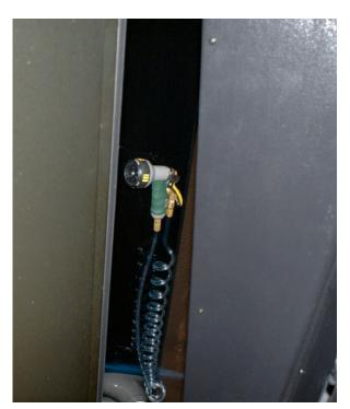
Rinse the filter using the wash down hose inside of the unit. Replace the filter with the foam side down.
