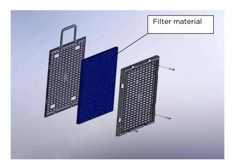
If the filter material needs replacing, unscrew the 4 screws on the EZ Fan Filter Assembly. This will remove the cover and allow you to replace the filter material.
