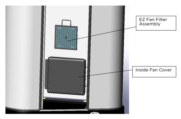
Grab handle and lift the fan filter assembly from behind the inside fan cover. Remove rinse and replace the filter.
