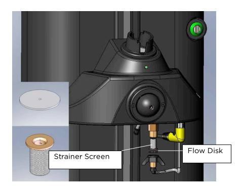
Remove and wash the flow disk and the strainer screen. Reassemble the liquid flow disk assembly, as shown. Tighten wing nut only hand tight. Do not over tighten.
