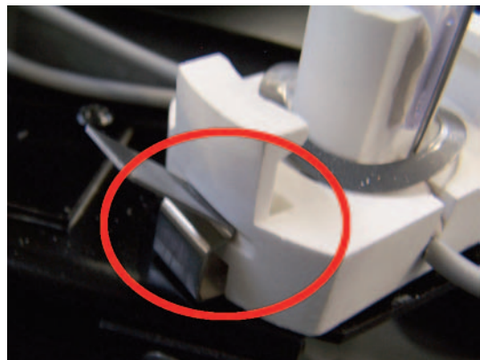
Illustr. 5-6-6: Insert the new burner and ensure a snug fit
