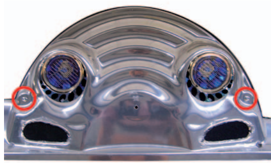
Illustr. 5-6-2: Undo the screws holding the chrome covering
