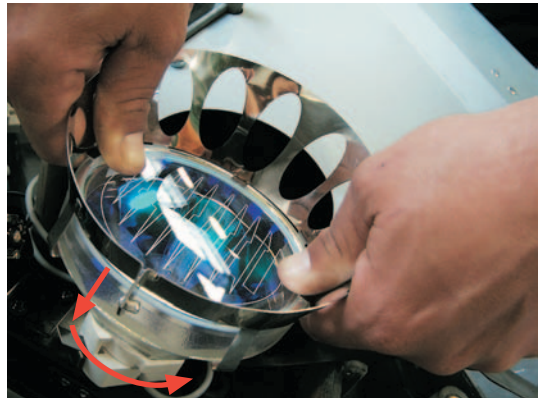
Illustr. 5-6-4: Unscrew the reflector
