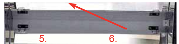
Abb. 3-8 Clamping springs retaining the filter panes
