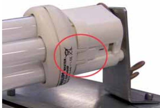
Fig. 3-6-7 Correct position of the connector
