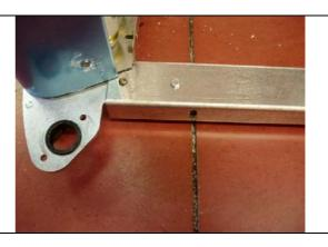
Connect panel5 to panel 2 inserting panel5 into long brackets as shown below, without completely tightening the screws.
