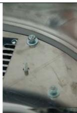
Insert plastic cylinders on the top side of panel 1 and 6 (doors);
